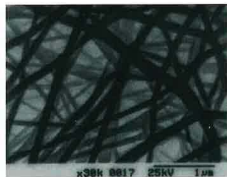
Fig.7 SEM photograph of CS/SER/PEO (8/2/2) nanofibers mat.
