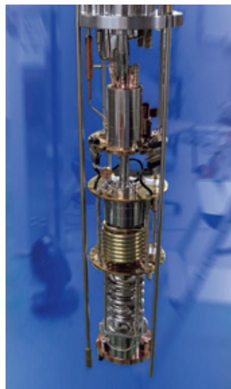
Fig. 2: 3 He / 4 He dilution refrigerator which can generate milli-kelvin temperature range.
