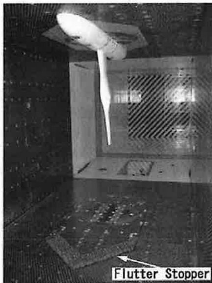
Fig. 8 Model installed in the wind tunnel test
