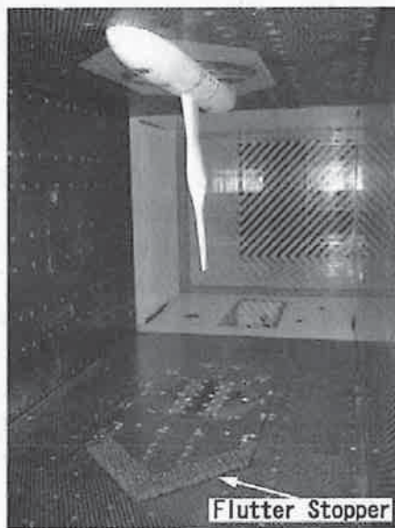
Fig. 8 Model installed in the wind tunnel test
