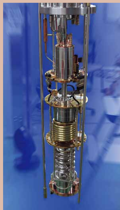
Fig. 2: 3 He / 4 He dilution refrigerator which can generate milli-kelvin temperature range.
